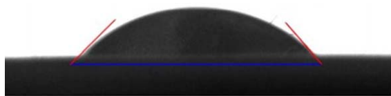
Figure 8. Contact angle of agarose/PAAm sheet. [Color figure can be viewed in the online issue, which is available at wileyonlinelibrary.com .]
